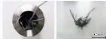
Chips remain in the hole
