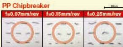
PP Chipbreaker controls chips stability at high feed rate.
