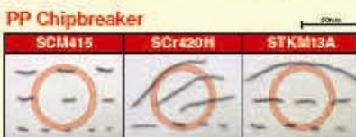
PP Chipbreaker controls chips stability from general steel to soft steel.
