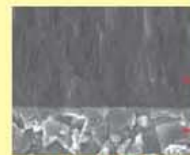
TiCN layer Carbide substrate
